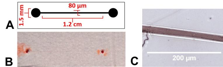
**Figure 2.** (A) Schematic of microfluidic device (Channel with a length of 1.2 cm, width of 80 μm and an injection port with a diameter of 1.5 mm). (B) Physical microfluidic device with red dye in order to ensure complete flow through channel. (C) Microfluidic device under brightfield microscope at 10x magnification.
