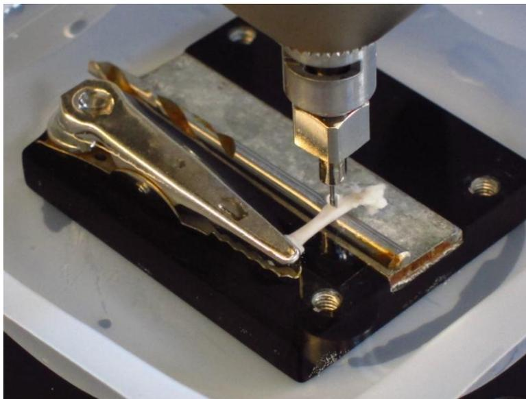
**Figure 3. The distal end of the femur is clamped to provide stability for testing and the probe assembly is lowered to rest perpendicularly on the bone, which is submerged in PBS with 1mM  $\text{CaCl}_2$ . A metallic rod is placed under bone such that it is aligned with the probe assembly.**
