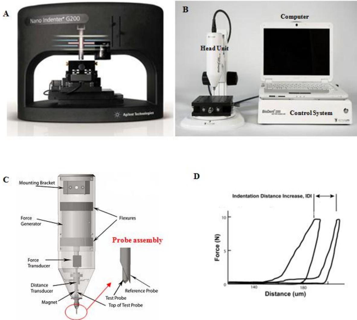
**Figure 2. (A) Nanoindenter G200, a commercially available indentation testing device ([www.google.com](http://www.google.com)). (B) Reference Point Indentation instrument that measures Indentation Distance Increase (IDI) ([www.activelifescientific.com](http://www.activelifescientific.com)). (C) [34] Head unit of the reference point indenter that provides housing for various elements that are illustrated. (D) [34] Force versus distance curves are used to quantify IDI.**
