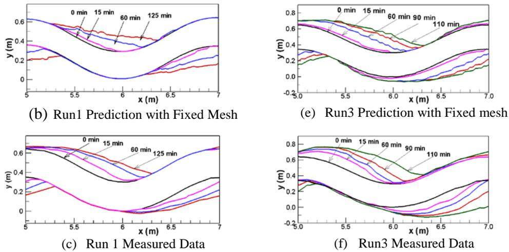
Figure 3. Comparison of predicted and measured bank retreat
