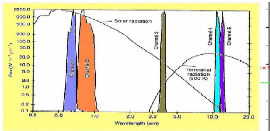
Fig. 2. Normalized spectral response of AVHRR
