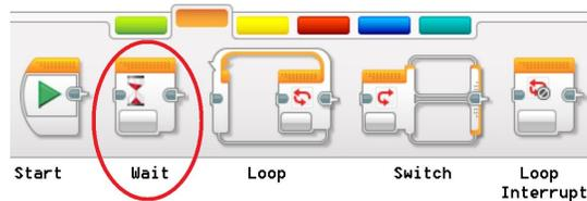
The image above shows an active orange tab in which the WAIT block can be found.
