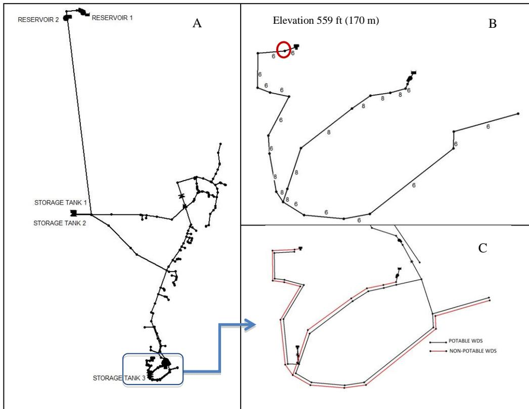
Figure 2. A. Potable and non-potable WDSs B. pipe sizes for non-potable WDS and simulated fire event location. C. The non-potable WDS.
