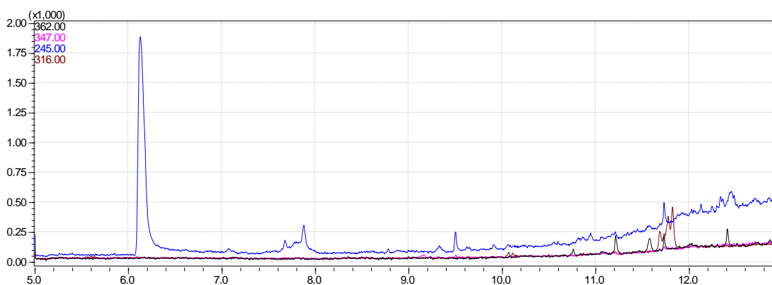
Fig # 8 Single ion monitoring chromatogram of m/z 362, 347, 245 and 316 of a blank synthetic urine sample injected after 2000 ng/mL calibrator.
