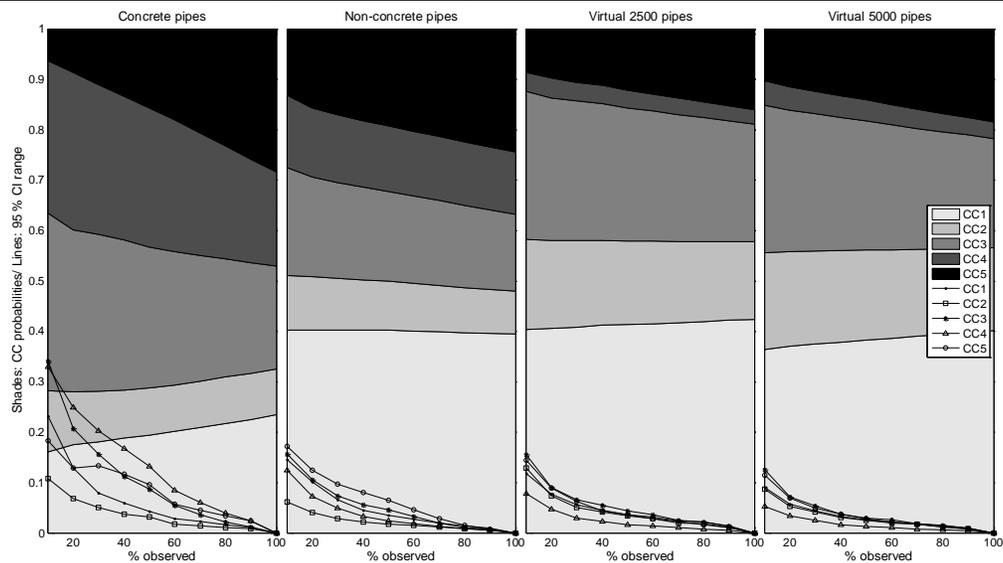
Figure 1. CC probabilities as a function of inspection rate (shades) and 95 % confidence interval range (lines)
