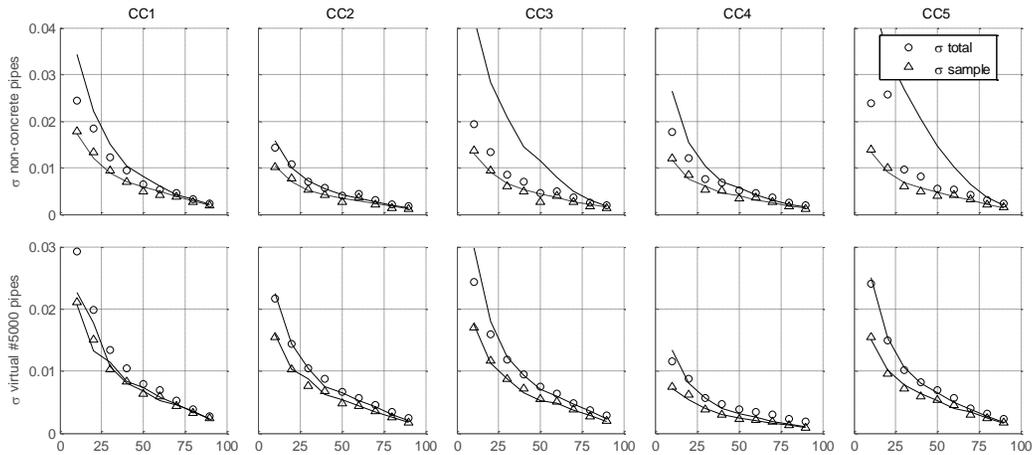
Figure 3. Comparison between standard deviation from Monte Carlo simulations (lines) and the uncertainty assessment method for incomplete datasets (points), as a function of the portion of inspected network. Sample and total standard deviations are shown.
