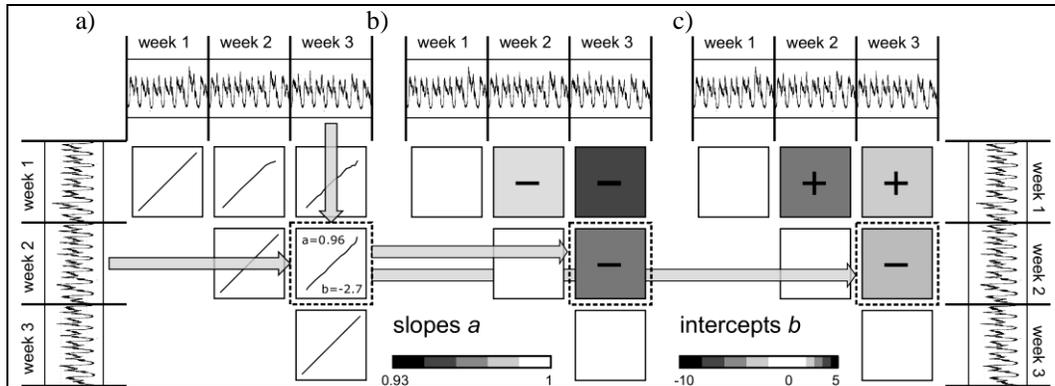
Figure 2: Illustration of the CFPD block analysis. a) CFPD analysis for each combination of blocks, b) visualization of slope values (matrix  $A$ ), c) visualization of intercept values (matrix  $B$ ). Copied from [2].
