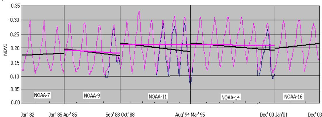
Fig. 8 New NDVI time series (weekly) (old NDVI data — , and new NDVI data — ).
