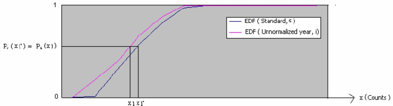
Fig. 5. Example of procedure to generate normalization data
