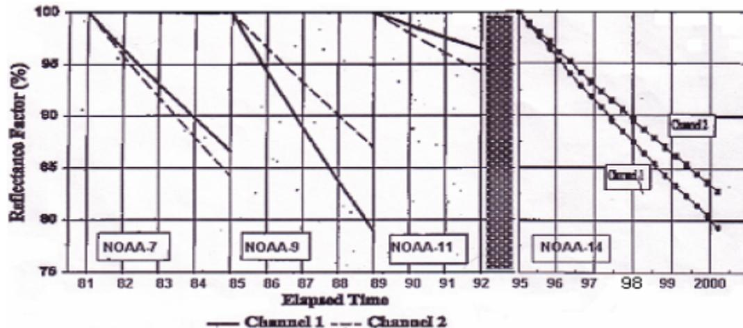
Fig. 3. Degradation of AVHRR Channels 1 and 2 [Rao, 1994]
