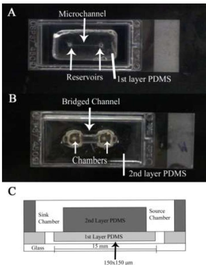
Figure 3: A) 1<sup>st</sup> layer of PDMS bonded to a glass slide. Two reservoirs are connected by a channel. B) 2<sup>nd</sup> layer of PDMS bonded to the first layer. A source and sink chamber align on top of the two reservoirs, and a bridge channel connects the two chambers. C) Schematic of the entire system, showing the dimensions of the channel.
