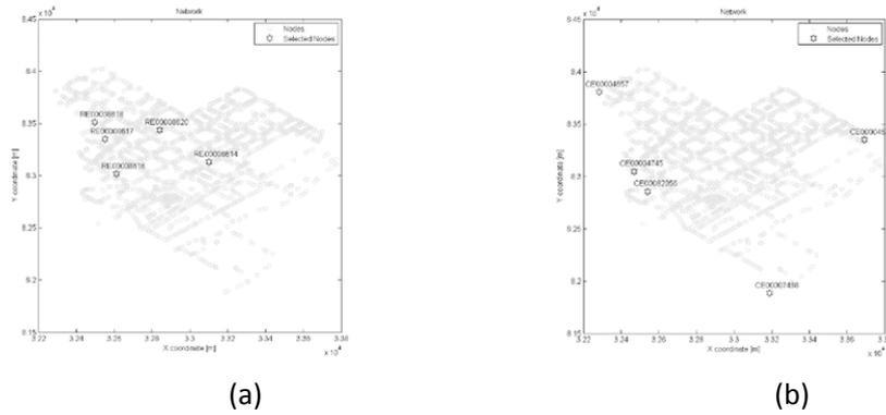
Figure 4. Pressure sensors in Nova Icària DMA, (a) Installed sensors; (b) Suggested demand sensitivity-based sensors
