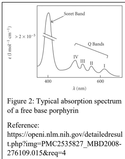
Figure 2: Typical absorption spectrum of a free base porphyrin
