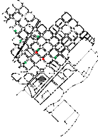
Figure 1 Water network of Nova Icaria DMA (EPANET model) highlighting inner pressure sensors (green stars) and DMA inlets (red triangles)
