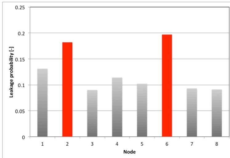
Figure 3. Posterior distribution of leakage probability in Scenario 2 (leaking nodes are in red)
