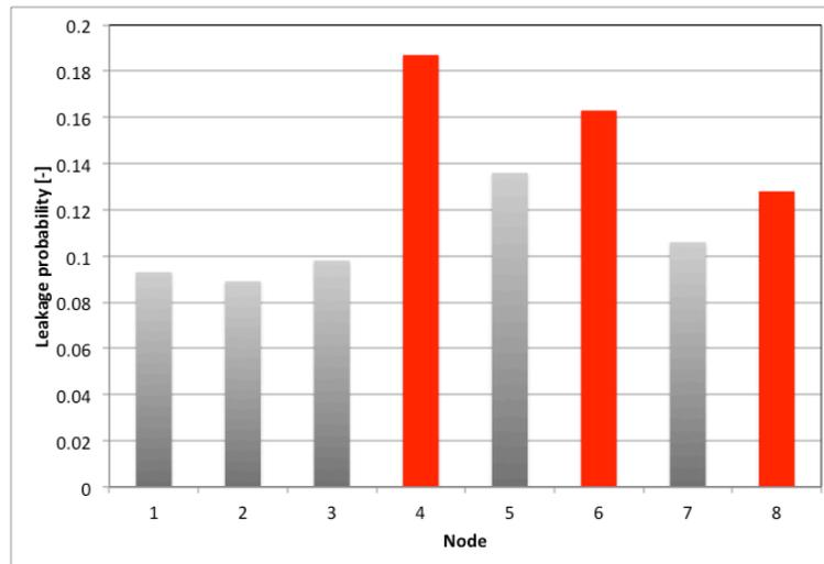
Figure 4. Posterior distribution of leakage probability in Scenario 3 (leaking nodes are in red)
