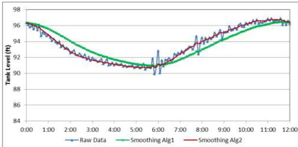
Figure 2. Example of tank level smoothing resulting using different algorithms
