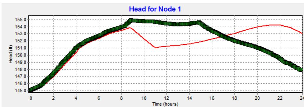
Figure 1. Example of model misbehavior with SCADA status operation only
