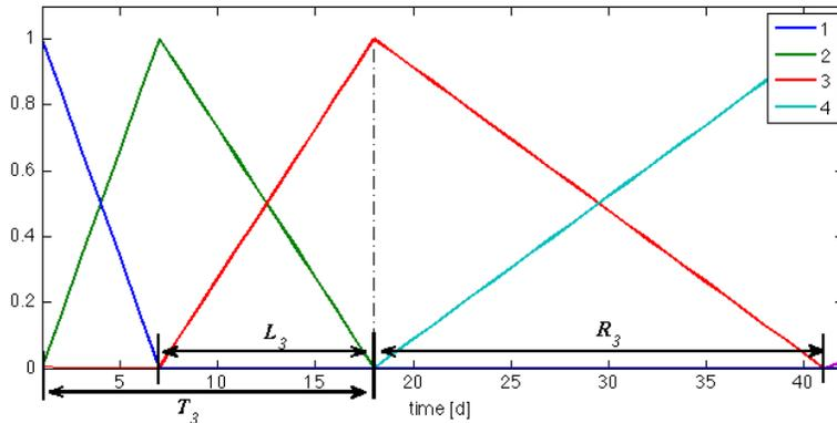
Figure 1. Example of basis triangular functions. For triangles 3, the peak time  $T$ , the left base  $L$  and the right base  $R$  are highlighted.
