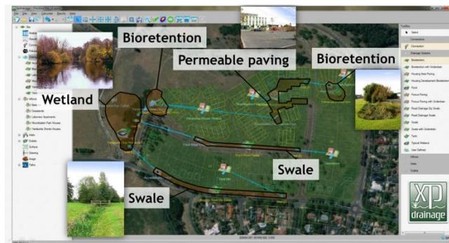
Figure 3. A drainage design modelled in XPDRAINAGE.
