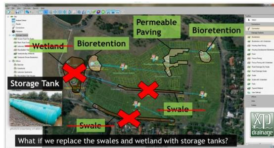
Figure 6. Modifying original design to include storage tanks.
