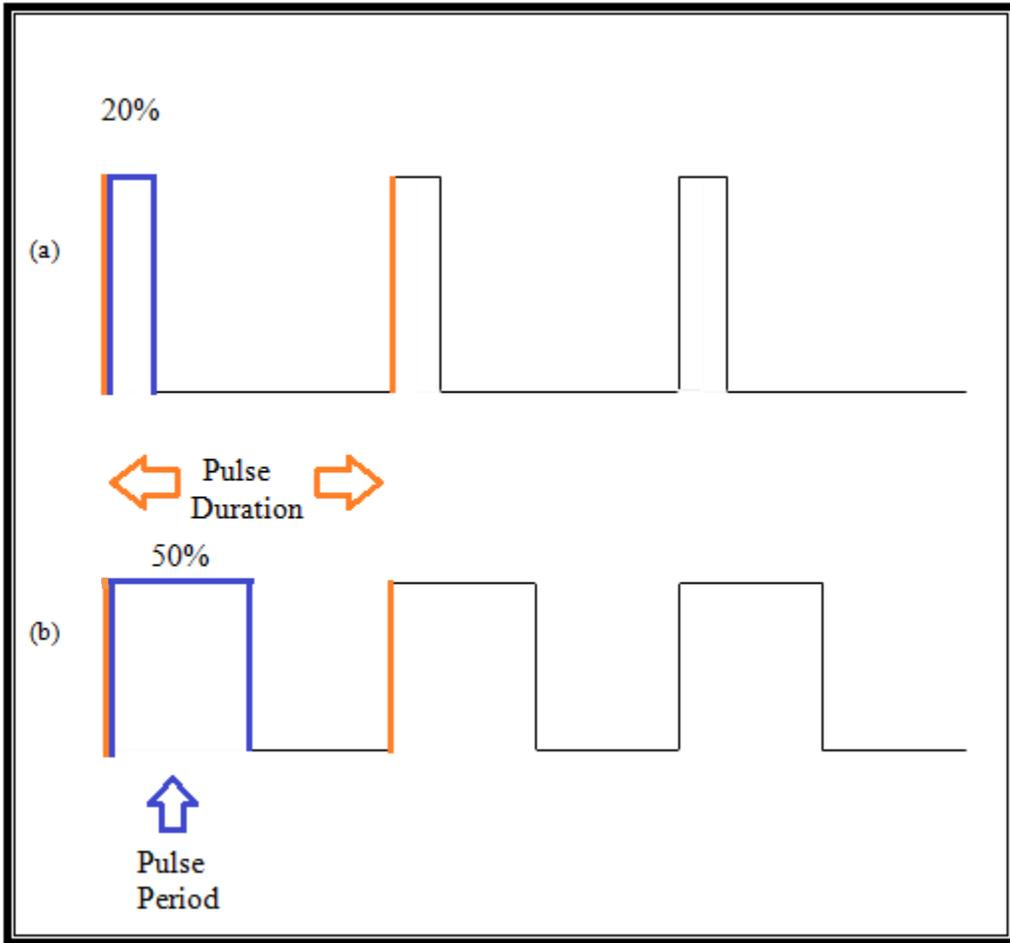
Figure 1. Illustration of (a) 20% and (b) 50% duty cycle. 20% and 40% duty cycle values were used in this experiment. (Adapted from Bar, 2001)
