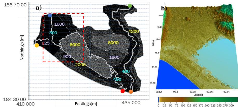
Fig 6. a) Illustration of the computational mesh utilised (numbers represent the maximum allowable area for an element within the region); b) LiDAR data (5m resolution) utilised for the definition of the topography.
