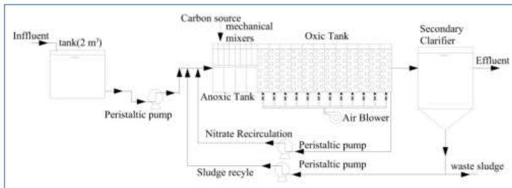
Figure 1. Schematic diagram of the pilot-scale pre-denitrification process
