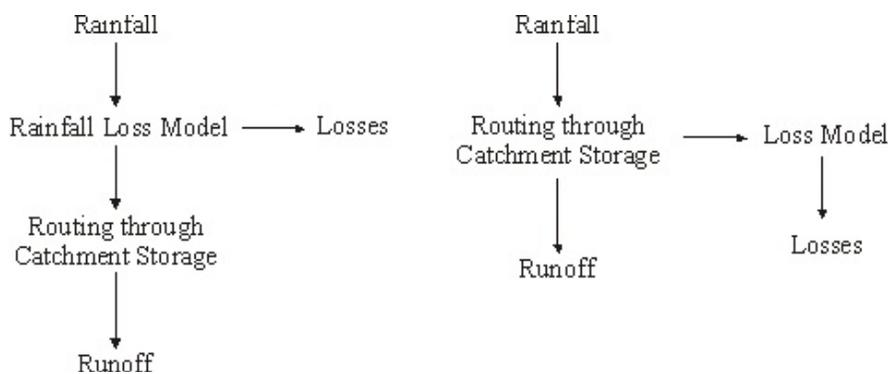
Figure 3. Alternative Rainfall Loss Models (after Ball *et al.*, 2011)
