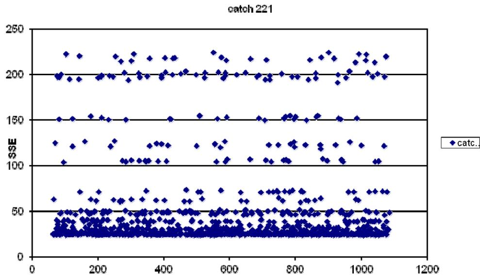
Figure 4. Variation in Sum Squared Residual with SWMM Width Parameter for 1 Subcatchment in a Catchment Model with 42 Subcatchments
