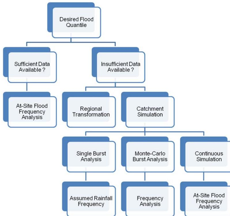
Figure 2. Design Flood Estimation Approaches (after Ball *et al.* [1])
