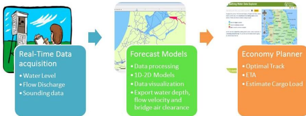
Figure 2. Schematized representation of FEWS-Waterways.
