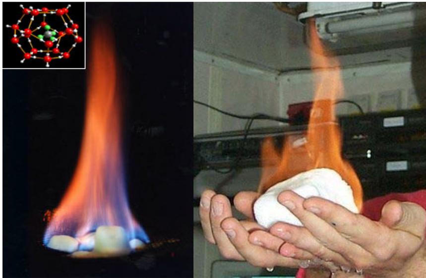
Figure 1: Burning methane hydrates [2].
