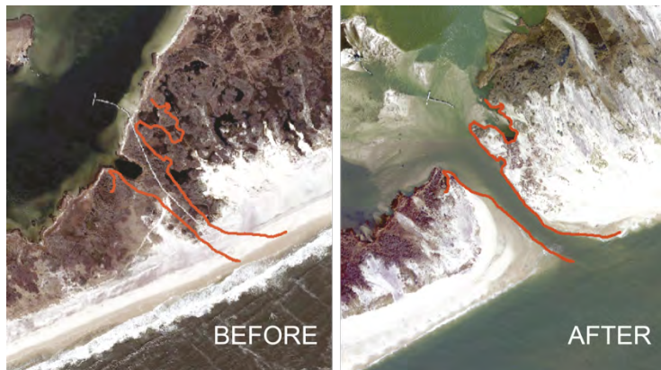
Figure 19. In 2012, hurricane Sandy pushed sand inland and cut a channel through the eastern end of Fire Island. The channel is still open today.
