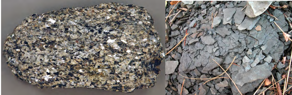
Figure 1. (a - left) The Manhattan schist from New York City and (b - right) a shale that is the parent rock or protolith for the schist. Figure 1a. by James St. John - Mica schist , CC BY 2.0. Figure 1b. by Pollinator , CC BY-SA 3.0.
