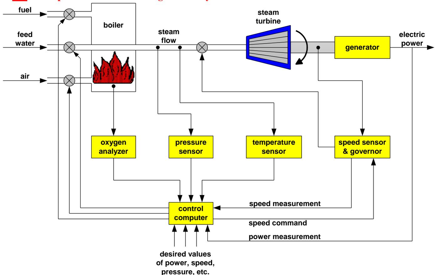
FIGURE 1.5 A computer-controlled multiple-input/multiple-output boiler-generator system, modified from Palm [1].
