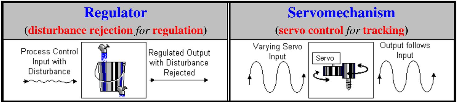
FIGURE 1.4 The role of control: regulator vs servomechanism.
