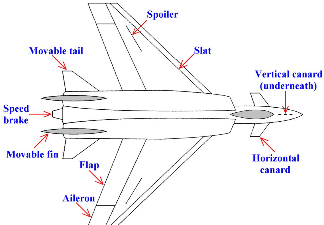
**FIGURE 1.10** A proposed futuristic control-configured aircraft, which utilizes more control surfaces than the usual elevators-ailerons-rudder system, modified from Palm [1].
