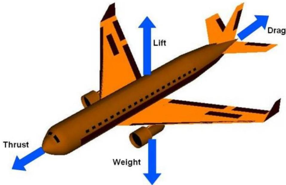
(a) **4** forces on an airplane: upward lift vs downward weight and forward thrust vs backward drag
