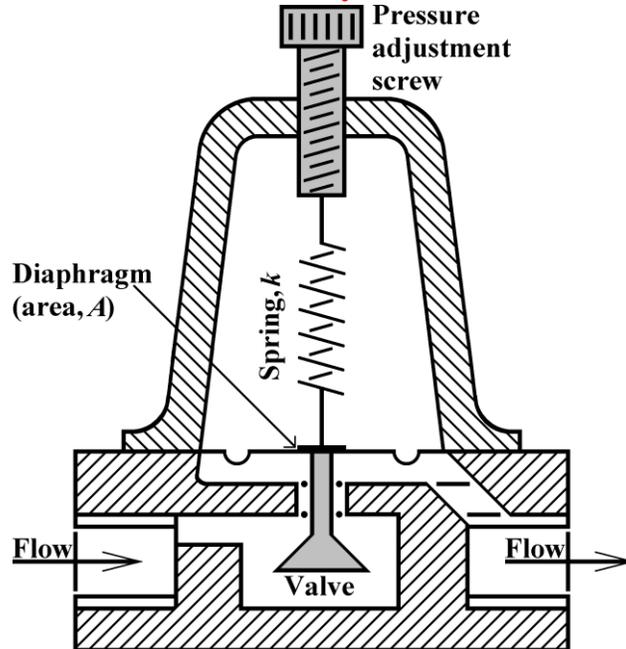
**FIGURE 1.6** A pressure regulator can be viewed as a component in a fluid level-flow system as well as a subsystem itself, composing of several components (flow-regulated valve, spring, diaphragm, pressure-adjustment screw, etc.), modified from Palm [1].
