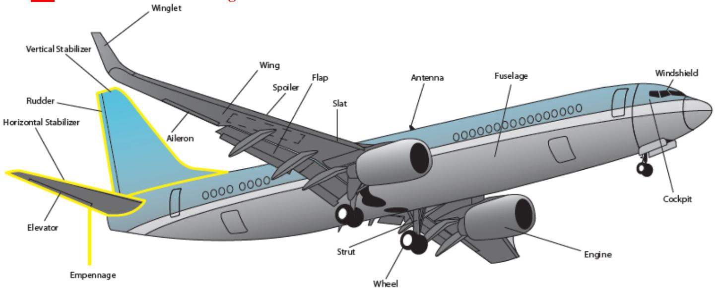
**FIGURE 1.7** Typical parts of a commercial airplane, adopted from NASA [2].
