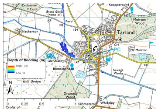
Figure 5. Flood inundation map of 1 in 2 year flow event with the storage pond at Netherton upstream of Tarland (Map reproduced by permission of Ordnance Survey).
