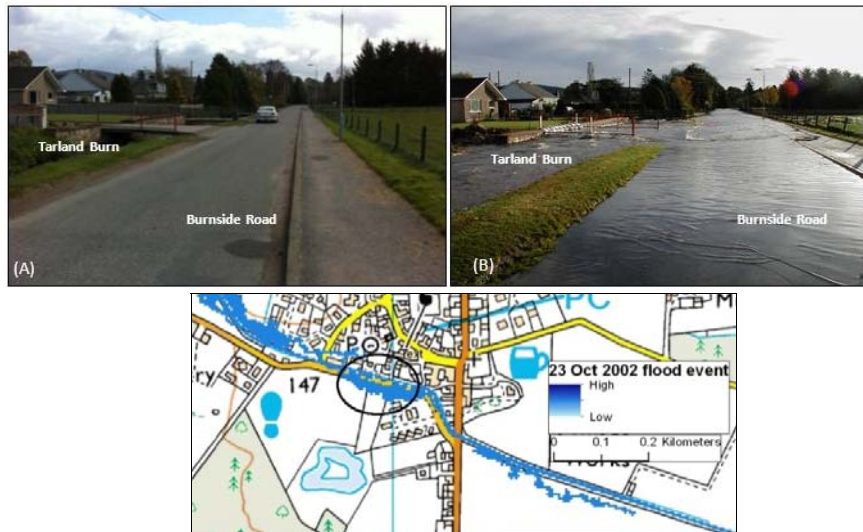
Figure 3. Bottom: Flood inundation map of October 2002 event. Top: (A) Normal conditions, (B) Flood conditions (Map reproduced by permission of Ordnance Survey).
