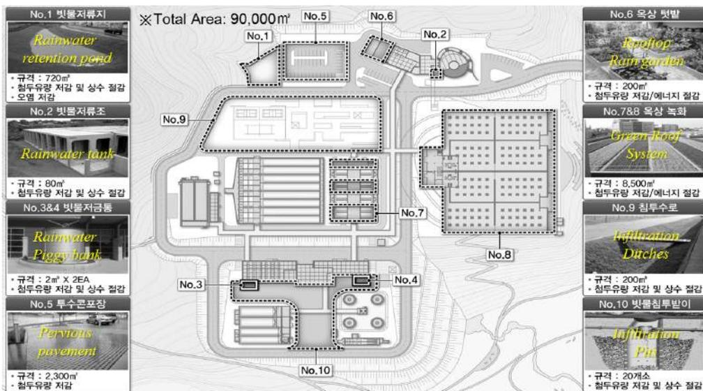
Figure 1. Installation map of 8 types rainwater facilities
