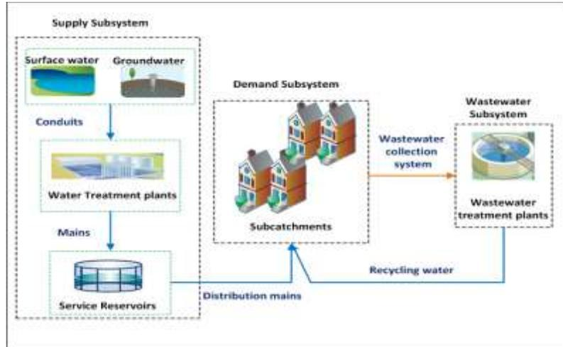
Figure 1. Main components modeled in an UWS
