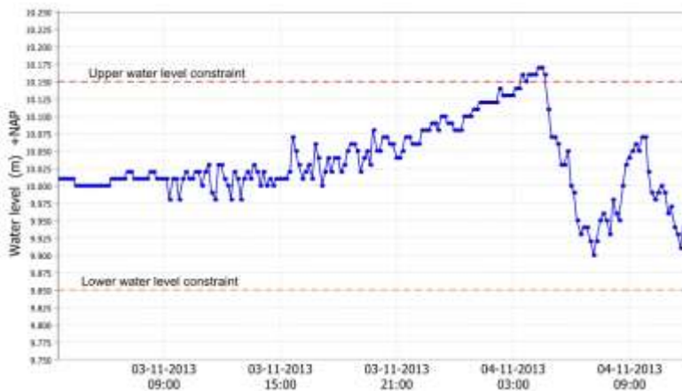
Figure 3 If a threshold crossing occurs during the night, the operator on duty receives an alarm signal and has to go to the lock to change the settings (data originates from the operational water management system).
