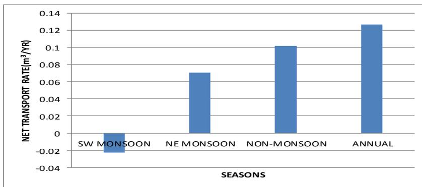
Figure 8. Bar graph of simulated net sediment transport in various seasons at Muthalapozy harbour.
