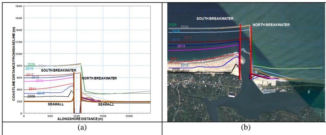
Figure 9. (a) Shoreline evolution from 2009 to 2029. (b) is superimposed on Google Earth image of year 2011 showing a match of the simulated results.
