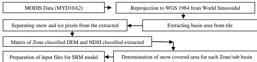
Figure 3. Preparation of snow cover input for SRM
