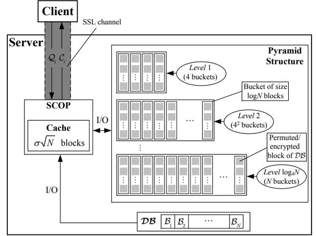
Figure 7: System architecture
