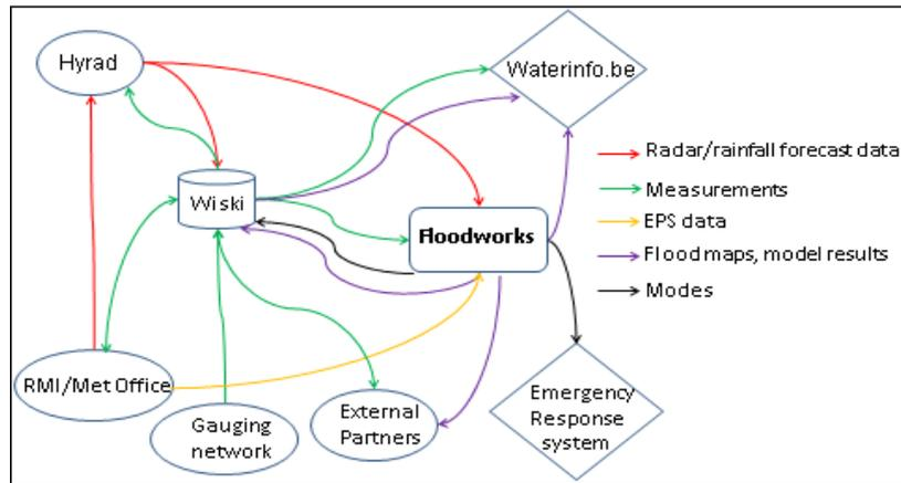
Figure 2. Dataflow of the flood forecasting system
