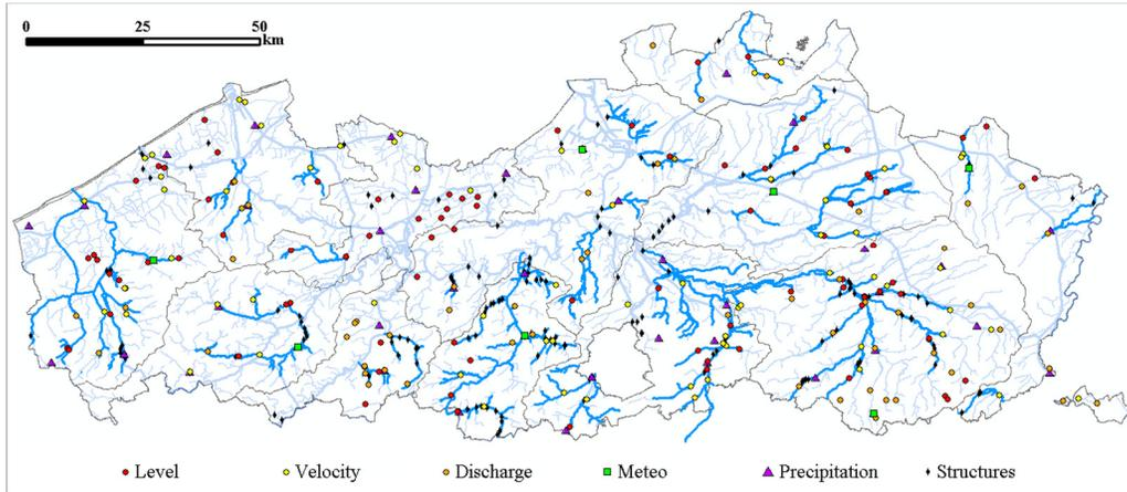
Figure 1. Extent of hydrodynamic models used in the operational flood forecasting system (blue lines) and overview of the gauging network operated by the Flemish Environment Agency
