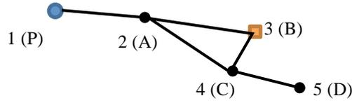
Figure 2. Example network model, with source node  $i=1$  (blue circle P), nodes where state variables are calculated  $n_n \in N_n = \{2,3,4,5\}$  and the observation node  $j=3$  (orange square B).
