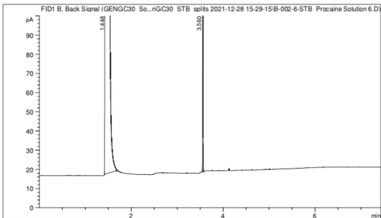
**FIGURE 14:** Procaine in MeOH Solution #6, Concentration – 0.052 mg/mL; Split ratio – 10:1
