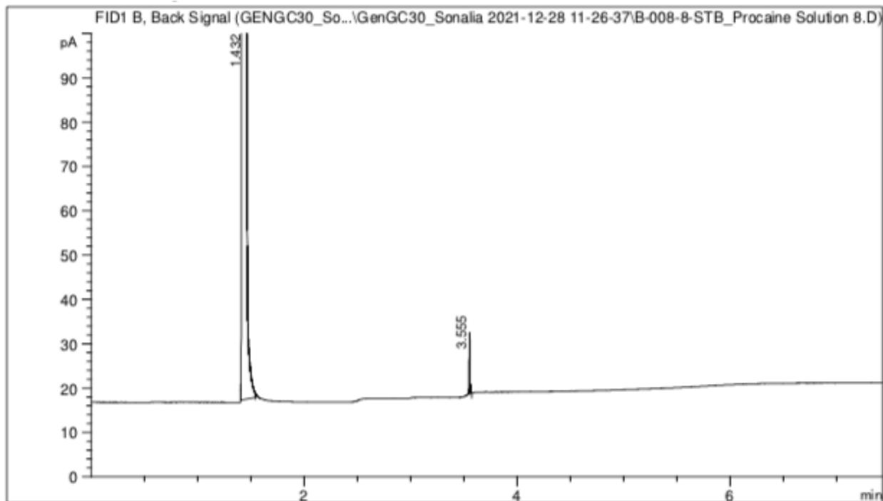
**FIGURE 11:** Procaine in MeOH Solution #8, Concentration – 0.031 mg/mL; Split ratio – 50:1
