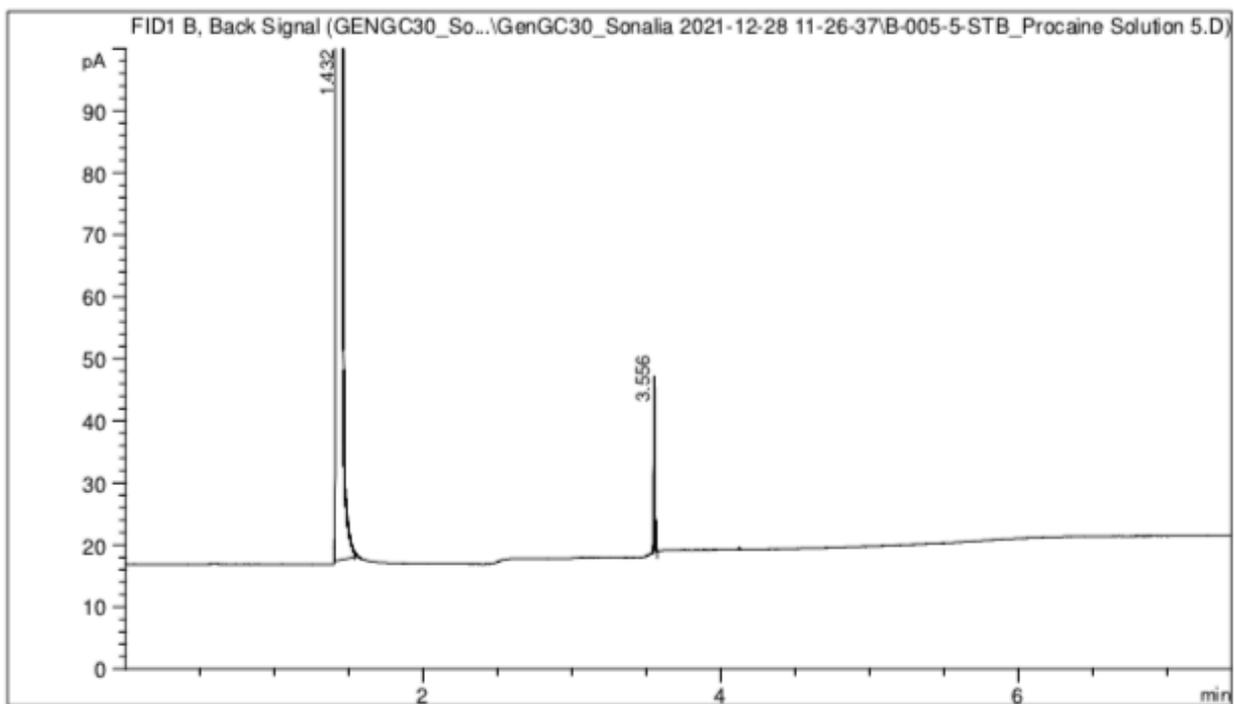
**FIGURE 8:** Procaine in MeOH Solution #5, Concentration – 0.062 mg/mL; Split ratio – 50:1
