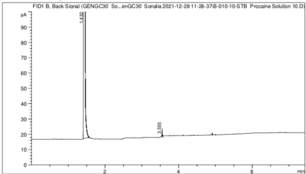
**FIGURE 13:** Procaine in MeOH Solution #10, Concentration – 0.010 mg/mL; Split ratio – 50:1
