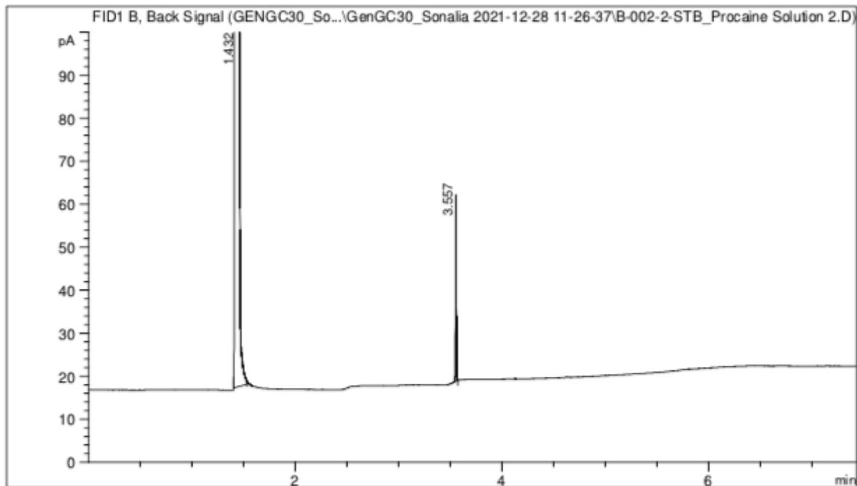
**FIGURE 5:** Procaine in MeOH Solution #2, Concentration – 0.093 mg/mL; Split ratio – 50:1
