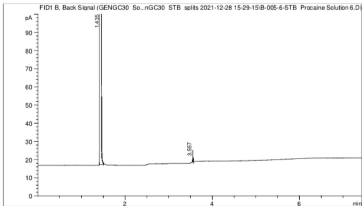
**FIGURE 17:** Procaine in MeOH Solution #6, Concentration – 0.052 mg/mL; Split ratio – 200:1
