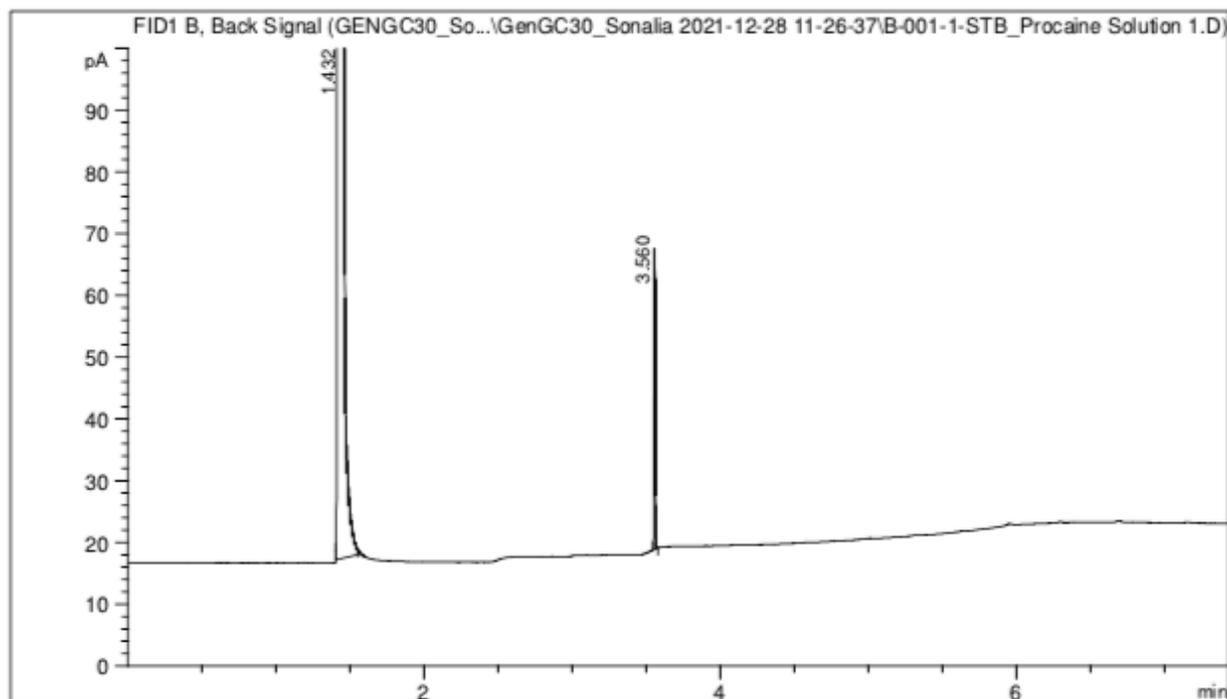
**FIGURE 4:** Procaine in MeOH Solution #1, Concentration – 0.103 mg/mL; Split ratio – 50:1
