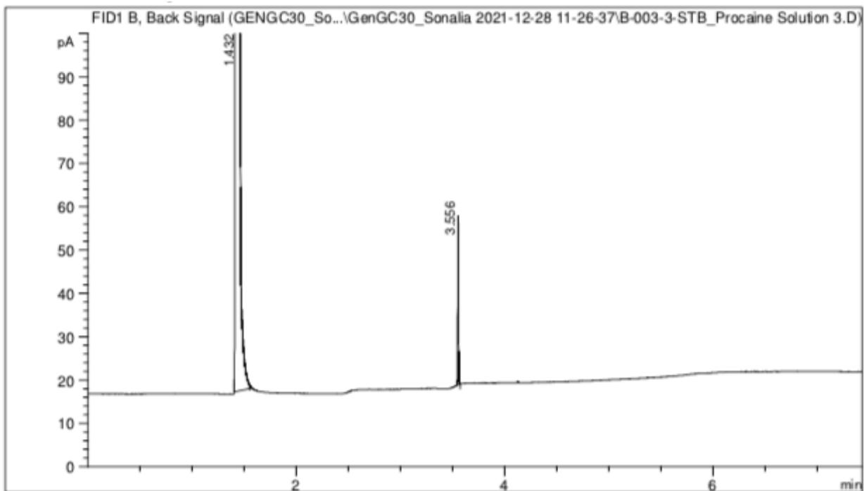
**FIGURE 6:** Procaine in MeOH Solution #3, Concentration – 0.082 mg/mL; Split ratio – 50:1
