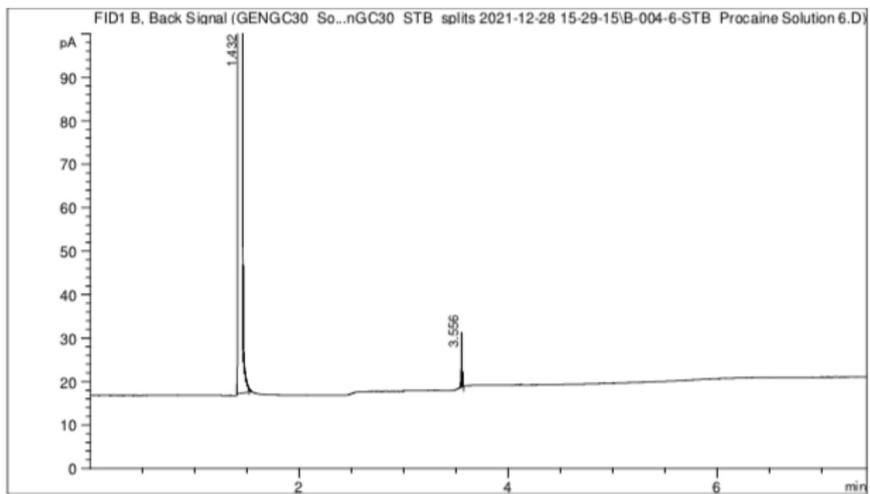
**FIGURE 16:** Procaine in MeOH Solution #6, Concentration – 0.052 mg/mL; Split ratio – 100:1
