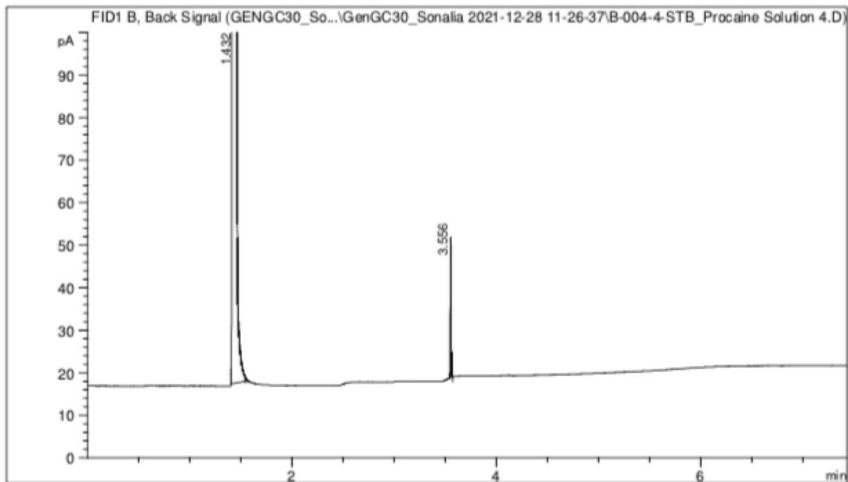
**FIGURE 7:** Procaine in MeOH Solution #4, Concentration – 0.072 mg/mL; Split ratio – 50:1
