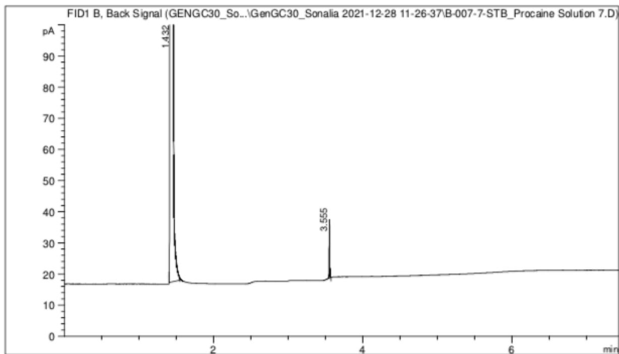
**FIGURE 10:** Procaine in MeOH Solution #7, Concentration – 0.041 mg/mL; Split ratio – 50:1
