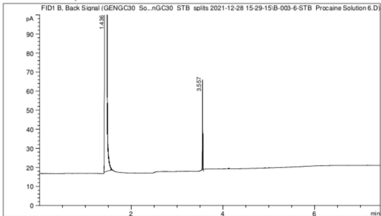
**FIGURE 15:** Procaine in MeOH Solution #6, Concentration – 0.052 mg/mL; Split ratio – 25:1
