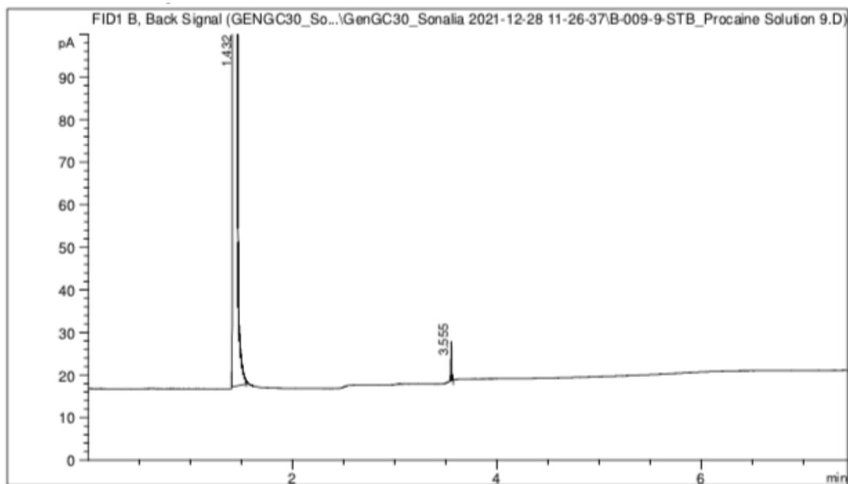
**FIGURE 12:** Procaine in MeOH Solution #9, Concentration – 0.021 mg/mL; Split ratio – 50:1
