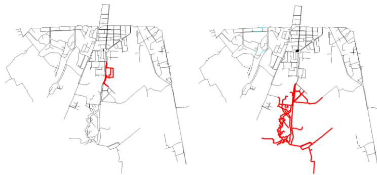
Figure 4. Set of probably leaky pipes in one of the most (left) and less (right) localizing clusters (result from the best Spectral Clustering).
