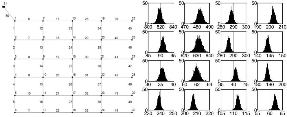
Figure 1.: Left: Network presented in [2]. We refer to the nodal demands as  $\mathbf{q}_{\text{Dem. Nom.}}$ . Right: Exemplary distribution of the flow rates due to random demand fluctuations as output of a Monte Carlo simulation.
