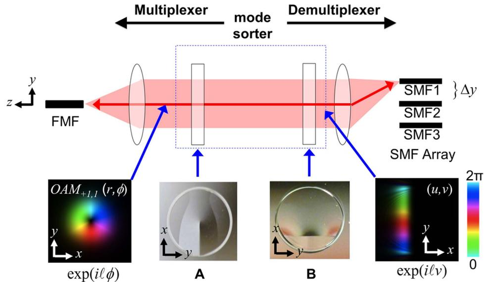
**Figure 1.** Concept of the OAM mode sorter. The OAM mode sorter functions as a mode multiplexer from right to left (SMF array to FMF), and functions as mode demultiplexer from left to right (FMF to SMF array). An OAM mode sorter consists of two custom refractive optical elements: (A) and (B).
