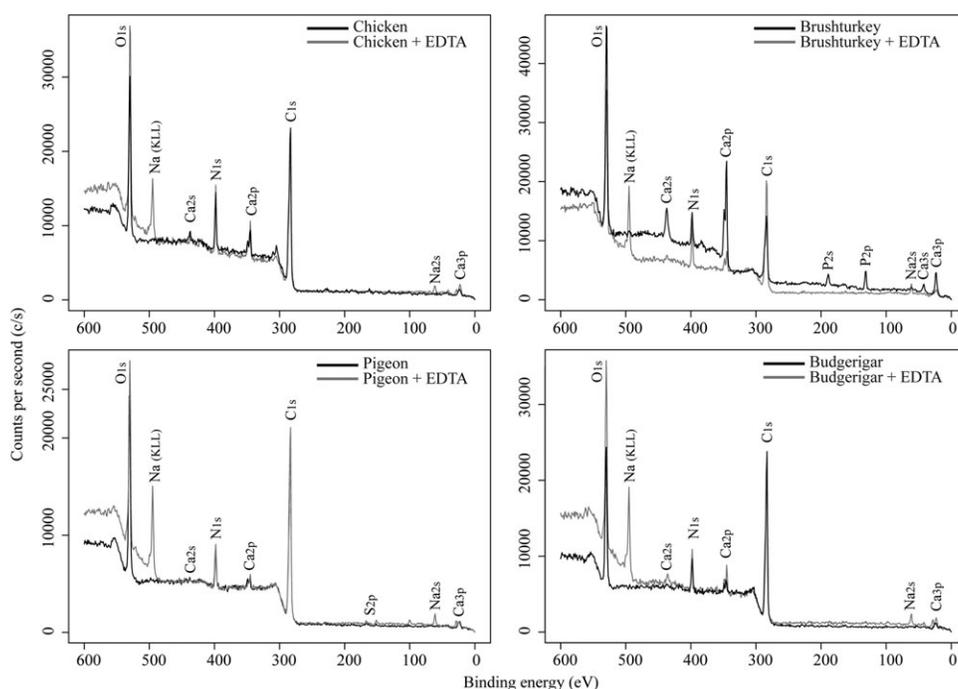
**Fig. 4.** XPS survey spectra showing the chemical composition of eggshells before and after EDTA treatment. The EDTA treatment duration are 90 min for chicken, brushturkey, pigeon, and 30 min for budgerigar. The sodium peak results from the residual presence of EDTA, and was not taken into account to calculate the atomic percentages.
