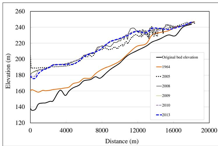
Figure 2 Longitudinal bed elevation of Shihmen reservoir
