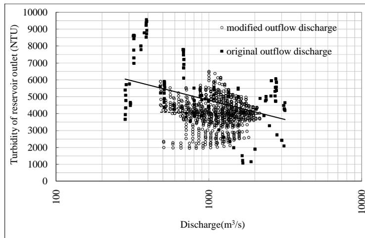
Figure 5. Effect of sediment concentration due to various outflow discharges of tunnel spillway
