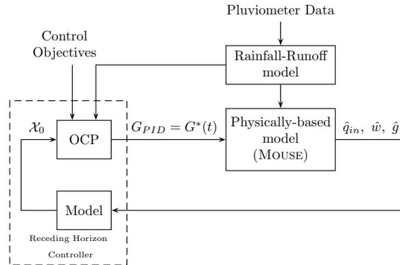
Figure 2: Diagram of the closed-loop simulation algorithm.
