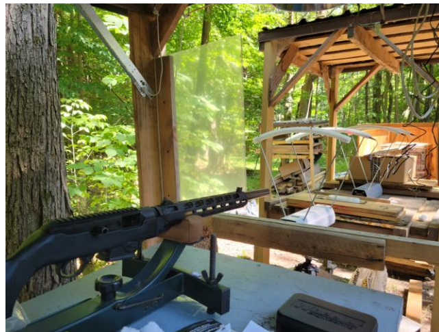
Figure 5. Set up for experiment with firearm in its rest, chronograph with infrared strips, and recovery boxes.
