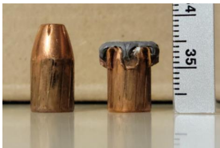
Figure 2. Side by side comparison of two fired hollow point bullets with no expansion (left) and full expansion (right).
