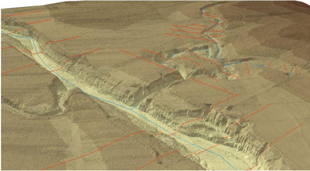
Figure 1. Example cross section and flowline geometry extracted from LiDAR terrain
