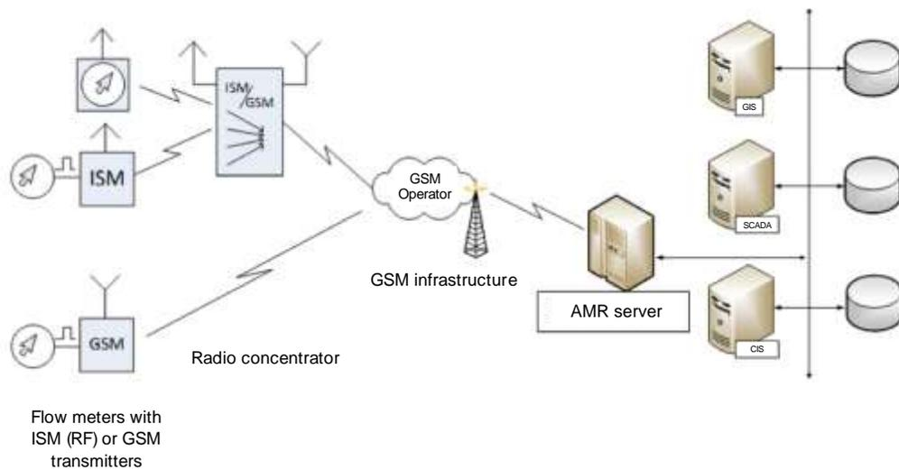
Figure 5. The automated meter reading system for Mikołów
