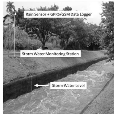
Figure 5. Details of storm water monitoring station
