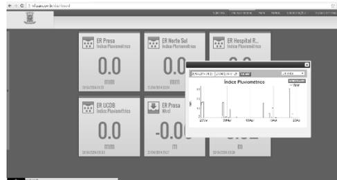
Figure 3. Dashboard of INFOSAN SaaS for monitoring data in real time.
