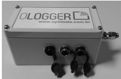
Figure 2. GSM/GPRS Datalogger with 3 input sensor and incorporated pressure sensor.
