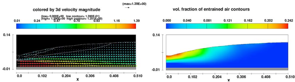
Figure 6. Velocity vectors and volume fraction in submerged hydraulic jump with FLOW-3D
