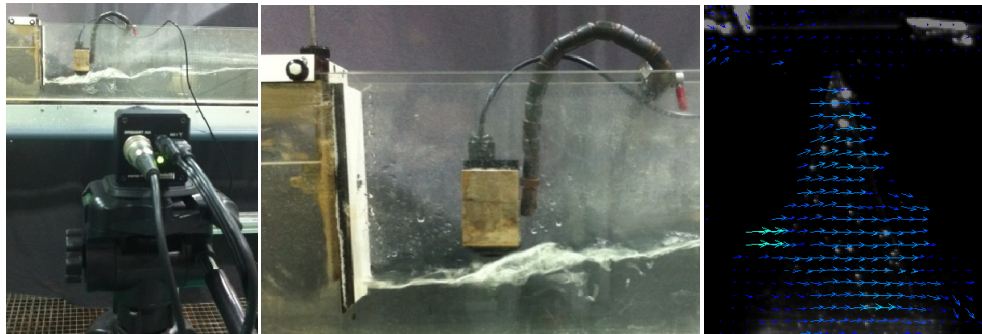
Figure 2. PIV instrumentation position and detail of post processing velocity vectors
