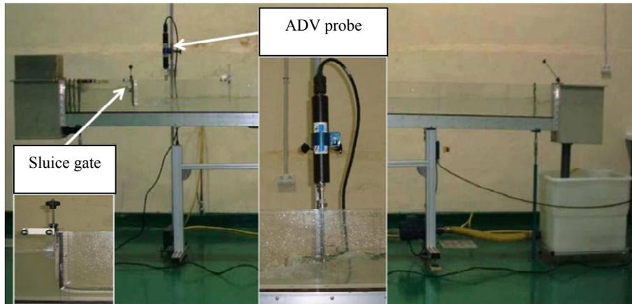
Figure 1. Free hydraulic jump at laboratory and acoustic Doppler velocimeter
