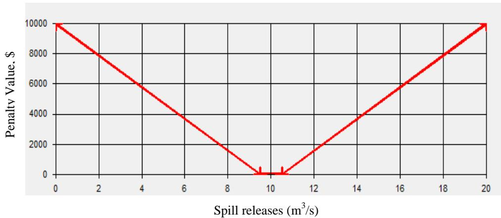
Figure 2: Example of a penalty function for spillway releases
