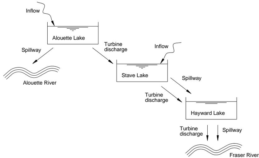
Figure 2: Hydraulic configuration of the Stave Falls project.
