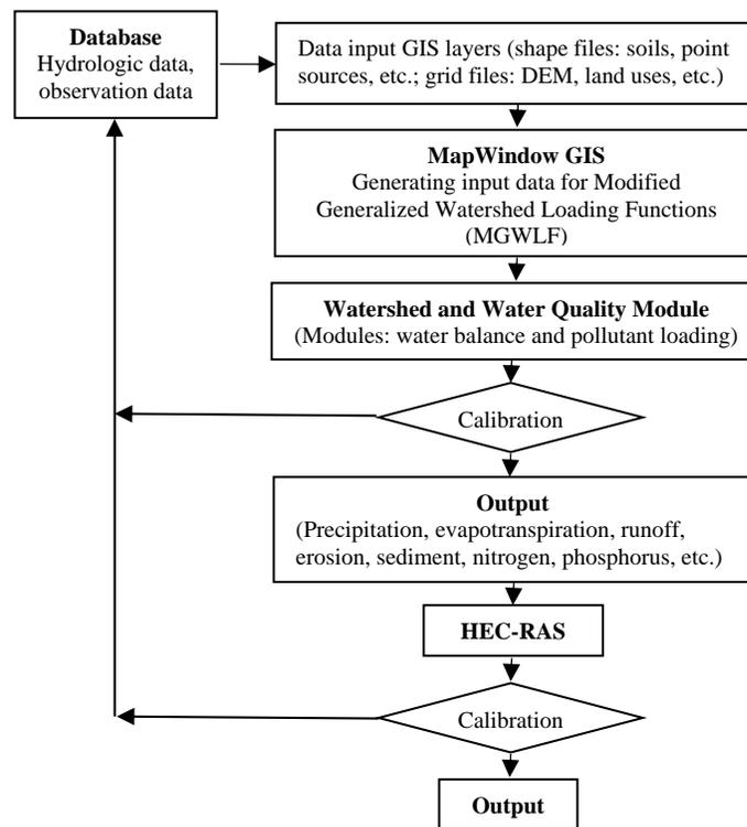
Figure 1. Scheme of the SNUWS model
