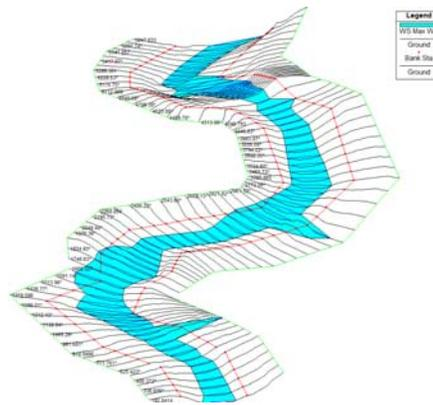
Figure 6. An interface with one-dimensional routing model, HEC-RAS
