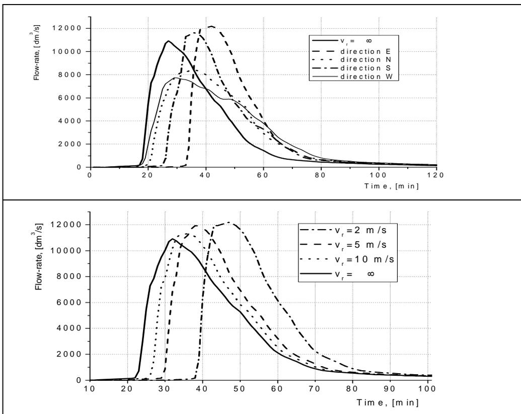
Figure 3a. Hydrographs for rainfall of duration  $t_d=20\text{min}$  ( $v_r=2\text{ m/s}$ ) for various directions of movement. Fig. 3b. Hydrographs for rainfall of duration  $t_d=20\text{min}$  (direction E) for various velocities.
