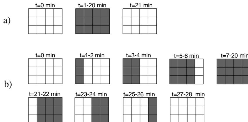
Figure 2. Scheme of rainfall movement over the catchment: a) static rainfall ( $v_r = \infty$ ), b) rainfall moving in east direction at speed of 5 m/s
