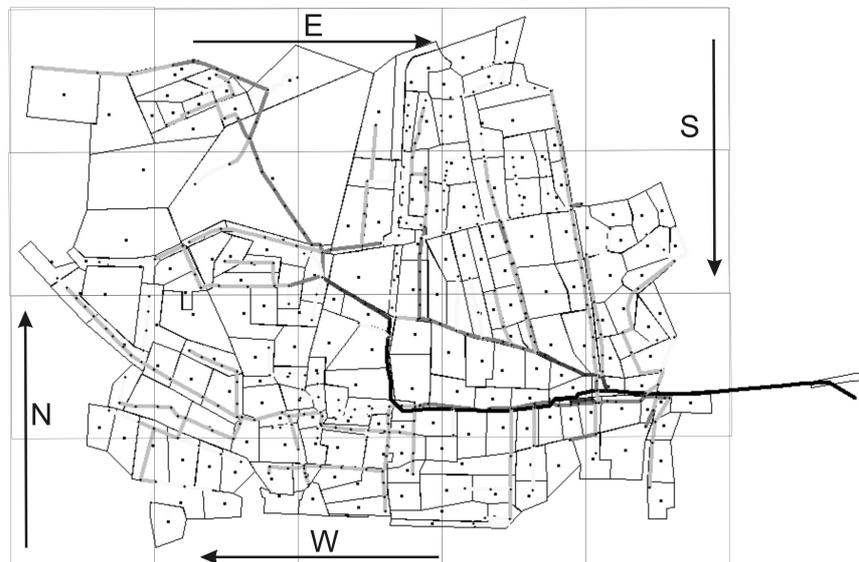
Figure 1. Scheme of modeled catchment divided on 200 subcatchments. Whole area divided into 16 sectors (dimensions 600x600m), which are the basis for simulation of rainfall movement over the catchment in four general directions (N, E, S, W).
